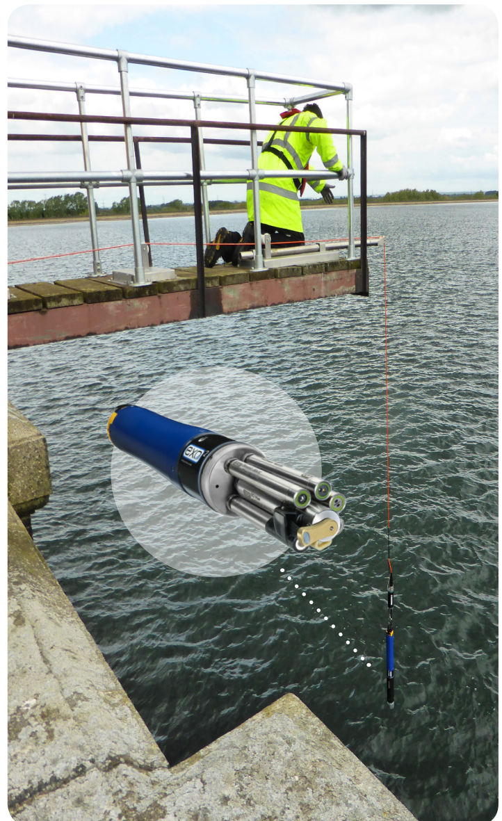
Fixed vertical profiling with a YSI EXO2 sonde.
