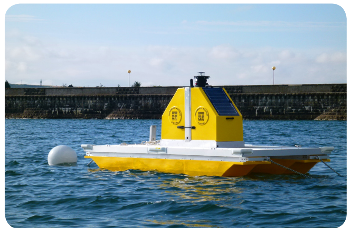
A YSI pontoon-mounted profiling system.
