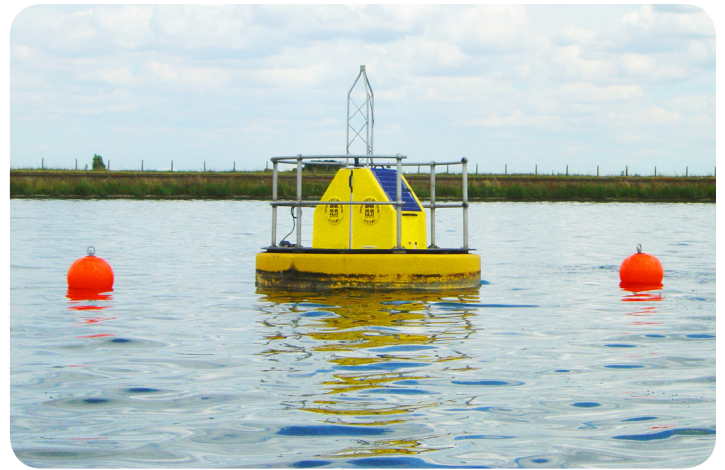
A YSI buoy-mounted profiling system.
